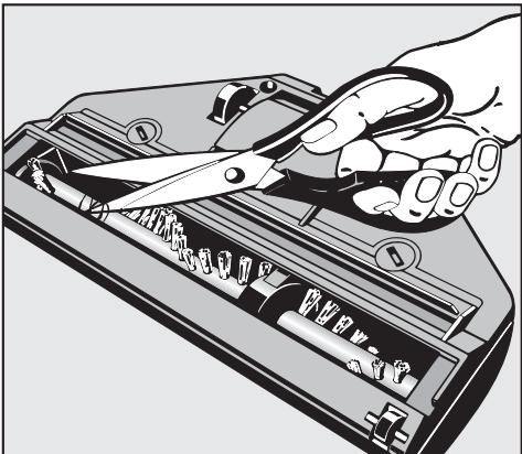
For more obstinate tangles or blockages inside the Turborbrush, the cover can be opened. Any large particles inside it can then be easily removed.
